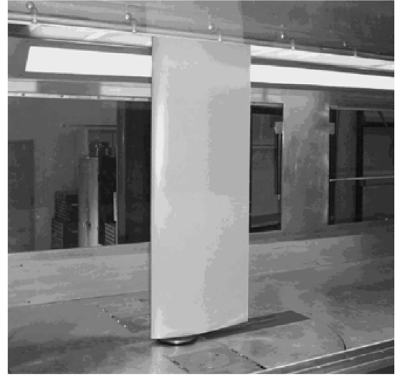
Fig. 2 A 2-D airfoil model, mounted in the UC Davis AWT test section.
